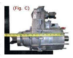
driveshaft would then need to be lengthened 3.0". This difference is now added to the measurement taken from your stock driveline, as recommended in the Preparation section. You would now have your new rear driveshaft length.
