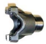
Yoke Modifications: Changing the style of yokes on the Atlas transfer case may require your new yoke to be modified. When installed on an Atlas, the yoke will load up against a tapered roller bearing. Some yokes require a chamfer to be machined to clearance the cage of this bearing. The yoke drawing shows the required machining on these yokes.
