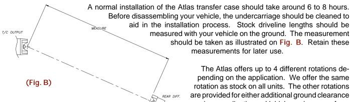
Before disassembling your vehicle, the undercarriage should be cleaned to aid in the installation process. Stock driveline lengths should be measured with your vehicle on the ground. The measurement should be taken as illustrated on Fig. B. Retain these measurements for later use.
