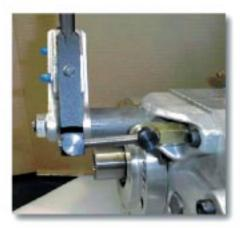
Atlas shifter problem check list: When installing the twin stick shifters, there are a few key areas that must be addressed. One of the most common difficulties we hear is that "my unit isn't shifting fully into one of the gear ratios". Incorrect adjustment of the shift handles to the linkage rods is normally the cause. With both shift rods in neutral, the linkage rod (connected to the shift handles) must be parallel with the aluminum shift tower. Refer to the photo left.
