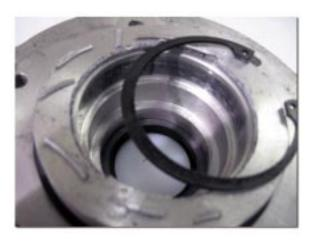
having been pre-loaded. Running the units in this state will cause complete destruction of the unit. In short, both units will need disassembly to fix the problem.
