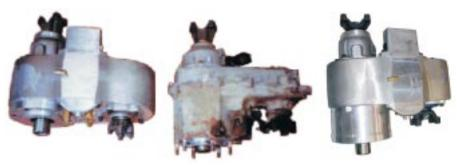
The Atlas 2 speed (left) & Atlas 4 speed (far right) in comparison to the NP231 (center) with a fixed yoke kit
