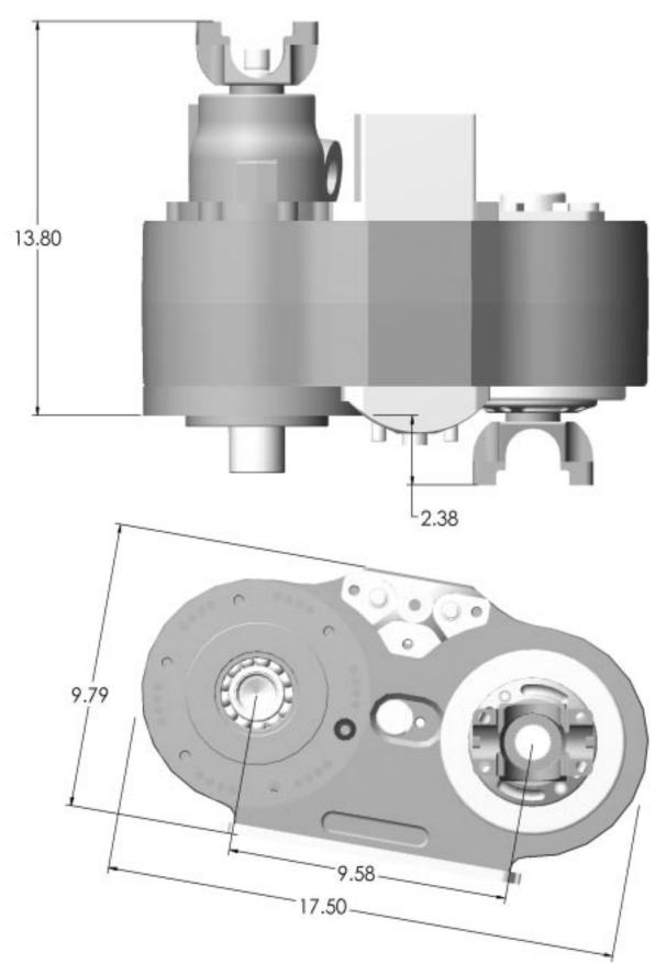
The Atlas measures approximately 14" from the center of the input to the outside edge of the main case. a TLAS 2 speed dimensions  $\frac{1}{2}$
