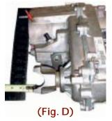
FRONT MEASUREMENT: Measure the stock transfer case from the front yoke face to the surface of where the transfer case bolts to the adapter housing (Fig. D). Write that measurement down.
